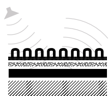
Regular hard or felt backed tile reflects more sound
